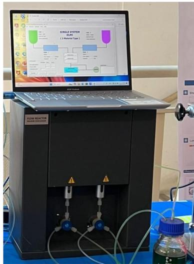
Gambar. Contoh reactor aliran mikro
